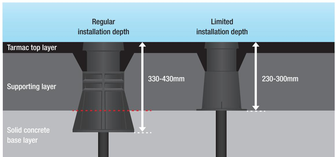
Since many years, AVK is one of the frontrunners in the development, production and sales of height adjustable surface boxes. A suitable solution for installation in tarmac.
