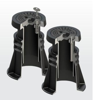
The so called suction effect that occurs when traffic passes over a surface box, can cause surface box lids to be lifted. By using AVK surface boxes with lid fixation, lids stay in place and unsafe situations are avoided.
